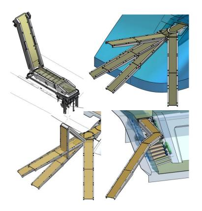
Standard Model: Available in either 510mm or 600mm built-in heights to accommodate varying reach requirements, ensuring compatibility with diverse yachts.
