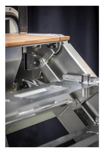
Step Width Options: Self-leveling steps available in widths from 1000mm to 2300mm.
