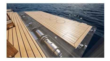
Maximum Load: Supports up to 14 kN·m of torque, with the option to combine multiple units per platform.
